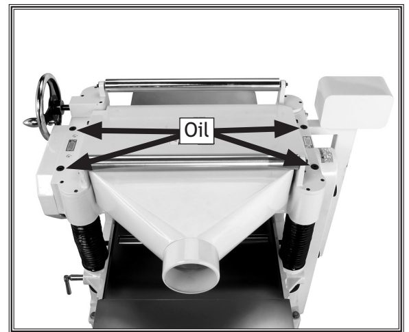
Figure 16. Feed roller lubrication locations.
